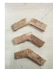
Fig:10- Tested sample with 30% fiber
