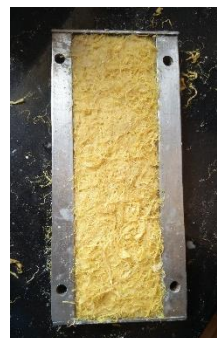
Fig:7- Fiber and Matrix placed in Die
