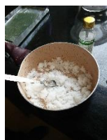
Fig:4- mixing of corn starch and glycerine
